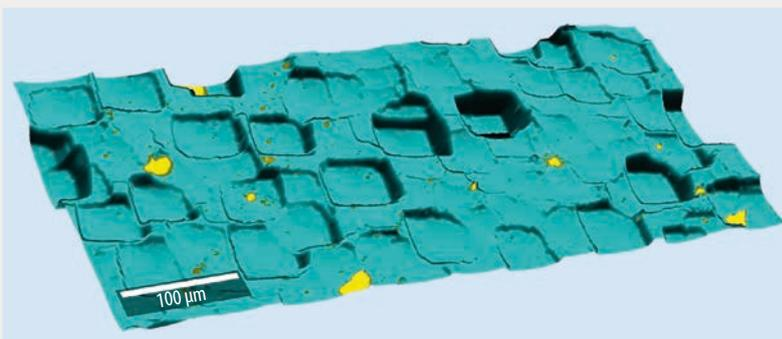
Topography and chemical composition of multi-crystalline silicon. Raman imaging reveals contaminants with increased fluorescence signal (yellow) on the silicon (turquoise). The topography was recorded by optical profilometry.
