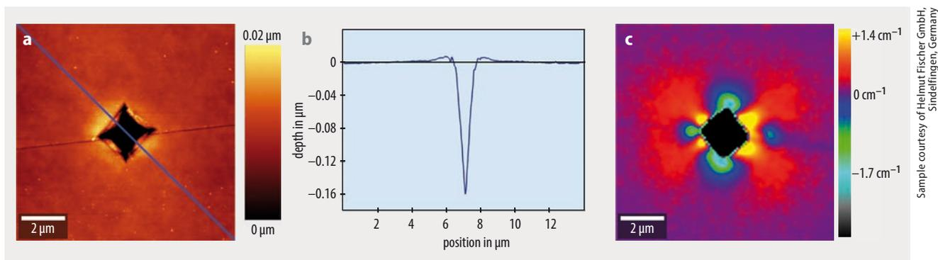
**Fig. 1** Characterization of topography and stress in silicon around a Vickers indent. AFM image of the topography around an indent (a),  $10 \times 10 \mu\text{m}^2$ . Depth profile along the blue line in the AFM image (b). Raman stress image of the same sample area as in (a) (c). The shift of the silicon Raman peak at  $520 \text{ cm}^{-1}$  is color coded.
