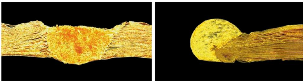
**Fig. 3** Welding of 34 stacked copper foils (each 11  $\mu\text{m}$ ) in butt welding (left) and edge welding configuration (right) with  $P = 580 \text{ W}$ ,  $v = 35 \text{ mm/s}$ ,  $df = 600 \mu\text{m}$ .
