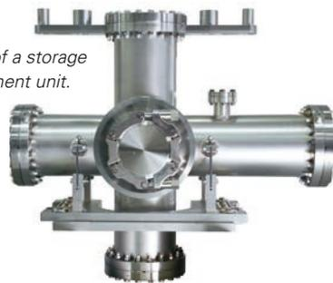
X-Y-Z manipulator with a differentially pumped rotary feedthrough for the positioning of samples in an ultra-high vacuum. The positions of the axes are read by encoders.
