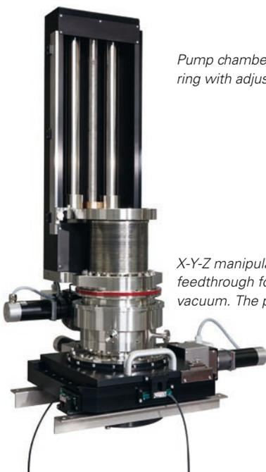
Pump chamber of a storage ring with adjustment unit.
