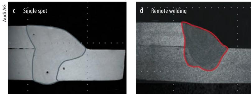
Fig. 4 Cross section of aluminum fillet weld lap joint
