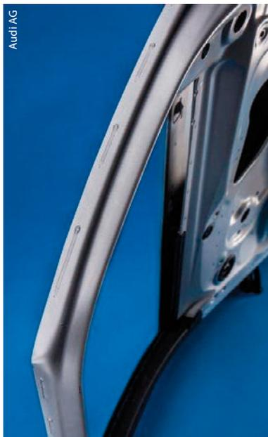
Fig. 2 Stitch and fillet welds in the Audi A6 aluminum door
