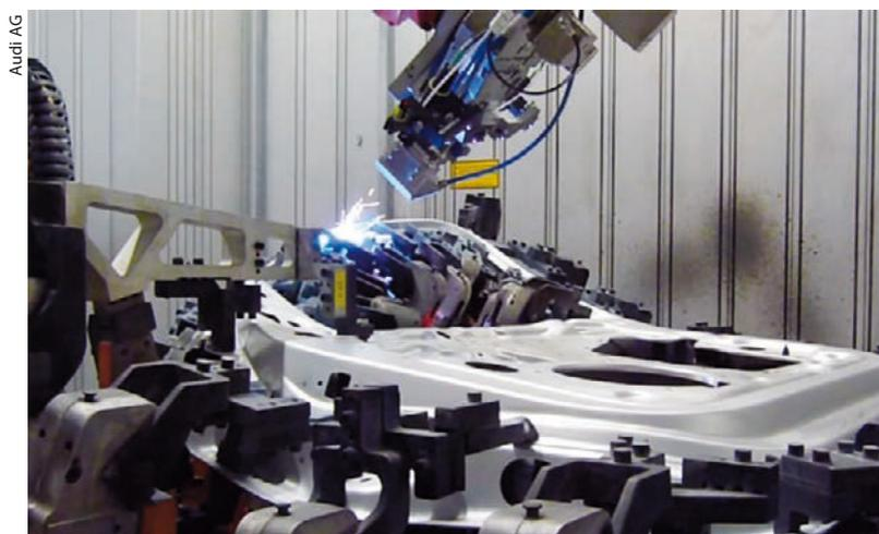
Fig. 5 Remote welding of Audi A8 doors
