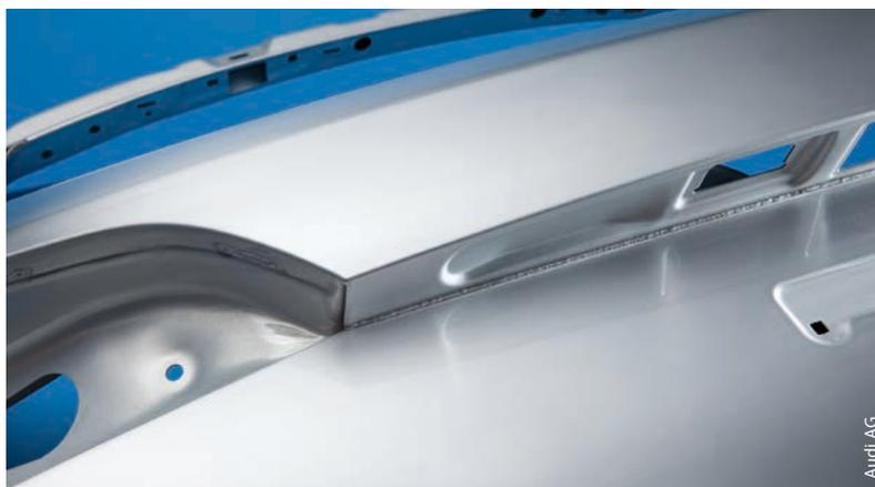
Fig. 1 Audi Q5 aluminum tailgate with weld seam in visible area
