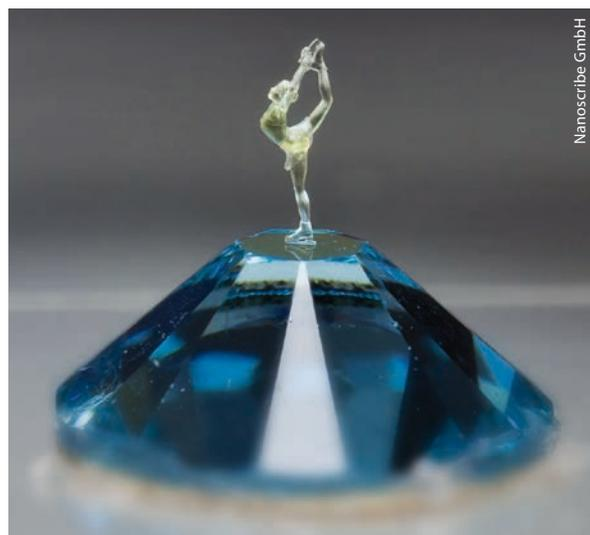
Fig. 2 With femtosecond fiber lasers of TOPTICA's FemtoFiber pro-series it is possible to produce extremely small three-dimensional structures. The shown figure has a height of about 3 mm, and is really standing on the blade of the ice skate. The applied process to generate such structures is a 3D-printing method which relies on two-photon polymerization (2PP). It uses the IP-S photoresist from Nanoscribe.
