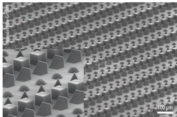
Fig. 3 The same method applied for the microstructure in Fig. 2 allows the fabrication of micro-optics with a size of only a few microns. Such small structures are particularly challenging for the lithography process and the applied components including the femtosecond fiber laser.
