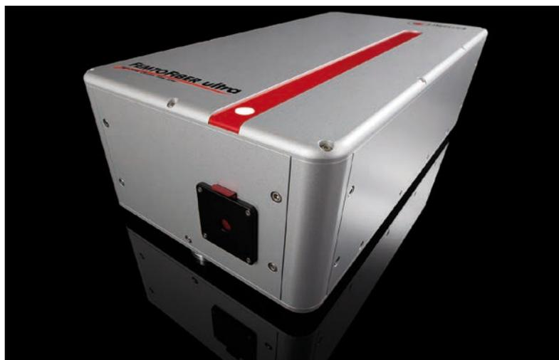
Fig. 4 TOPTICA's recent FemtoFiber ultra NIR is a femtosecond fiber laser that provides pulses at a central wavelength of 780 nm with a pulse duration of 150 fs at 80 MHz and an output power above 500 mW.
