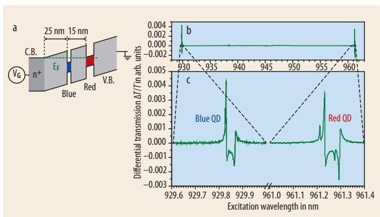
Fig. 4 a) Schematic band-edge diagram of a coupled double quantum dot. The wavelength-dependent differential transmission signal  $\Delta T/T$  of such a system is shown in b). It was recorded by a single
