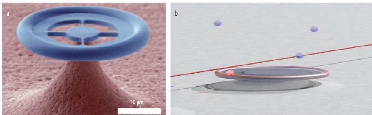
Fig. 3 a) Electron microscopy image of a microcavity that was used to demonstrate parametric coupling between light and this mechanical oscillator [1].
