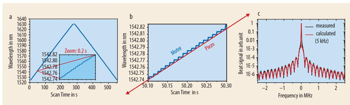
Fig. 2 a) Mode-hop-free wavelength tuning over 100 nm is enabled with the active SMILE stabilization of the CTL 1550. b) Motorized wavelength tuning can be performed with step sizes of
