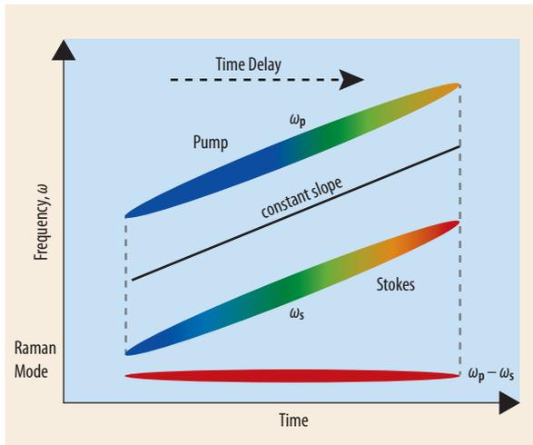
Fig. 3 Chirped CARS (spectral focusing) process. Constant slope gives narrow and constant frequency difference ( $\omega_p - \omega_s$ ) and center tuning aids selection of vibrational modes, which can also be achieved by temporal delay.
