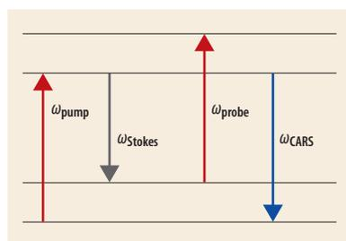
Fig. 2 In this CARS diagram both pump and probe wavelengths are the same. The CARS signal appears at the wavelength  $\omega_{\text{CARS}} = 2\omega_{\text{p}} - \omega_{\text{s}}$ .
