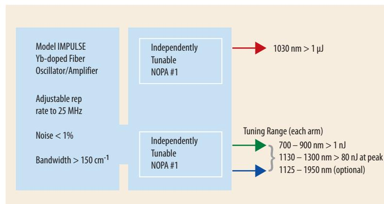
Fig. 4 Schematics of Model cOPA. Model IMPULSE pumps two NOPAs/OPAs giving two independently tunable, synchronized outputs. A synchronized, residual
