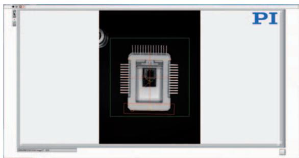
Fig. 5 Integrated image processing supports chip alignment prior to assembly (chip by STMicroelectronics).
