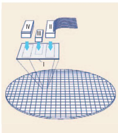
Fig. 2 Chip packaging: silicon substrate (I), fiber connection (II), external laser source (III) and flip-chip bonds (IV).
