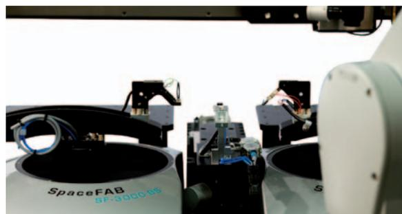
Fig. 6 Exact alignment of the optical fibers on a silicon photonic chip package using two SpaceFab positioning systems.
