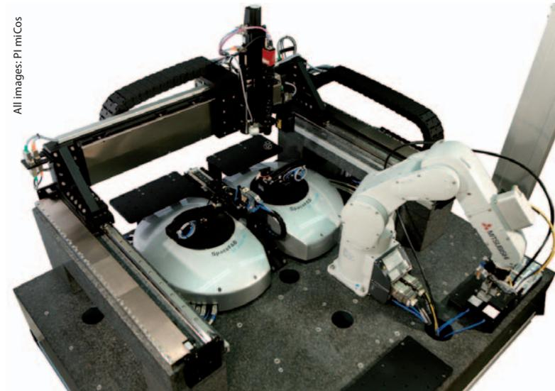
Fig. 1 Automated solution for silicon photonic chip production and inspection: the system integrates several hardware components and software for the automation of assembly and alignment, such as pick-and-place robot technology,
