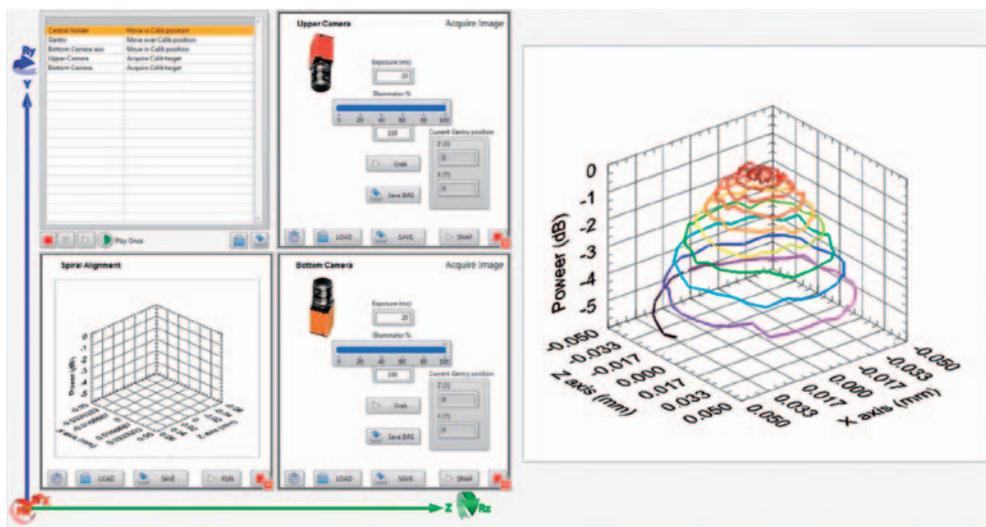
Fig. 4 Fine adjustment for fiber array: The light throughput is measured and optimized via scan algorithms.
