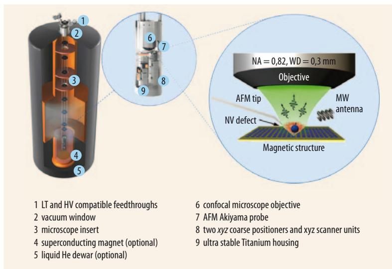
Fig. 1 Schematics of the combined atomic force and confocal microscope with
