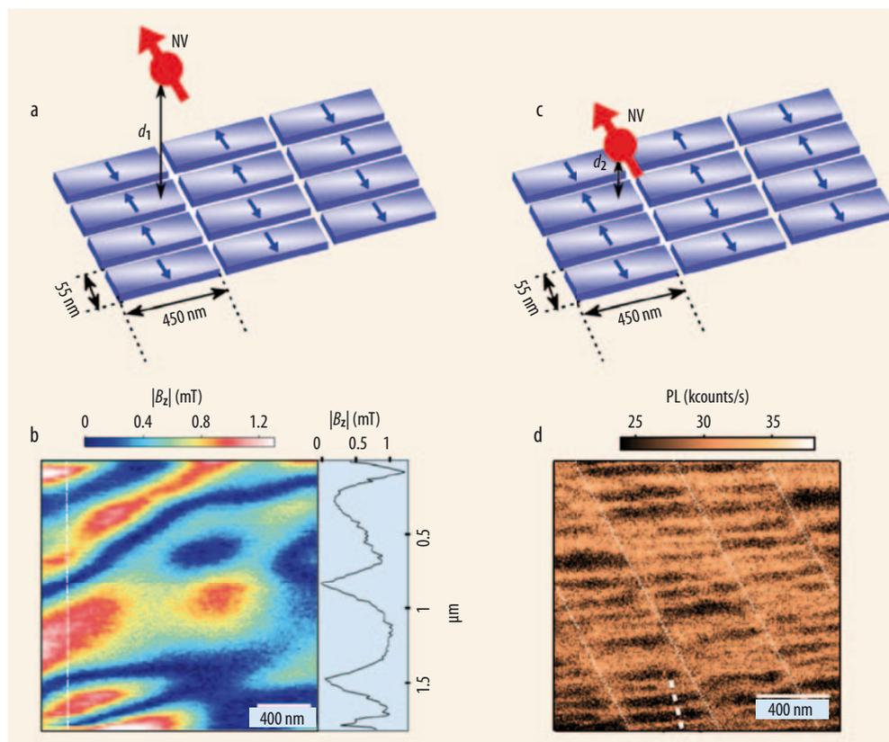
**Fig. 2** Here are two examples for magnetic imaging of a hard disk sample with random bit orientation: Quantitative imaging using ODMR based method with NV-center scanned at  $d_1=250$  nm above the sample (a) yields a quantitative magnetic field distribution (b) recorded with the lockin technique (13-nm pixel size, 110-ms acquisition time per pixel). The frame on the right shows a line-cut taken along the dashed white line in the image.
