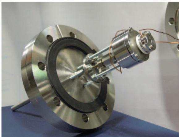
Fig. 4 The piezo-actuated pulsed valve
