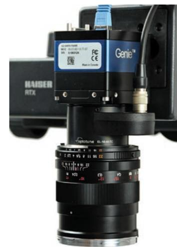
**Fig. 5** The Optotune Model EL-16-40 installed between camera and objective lens
