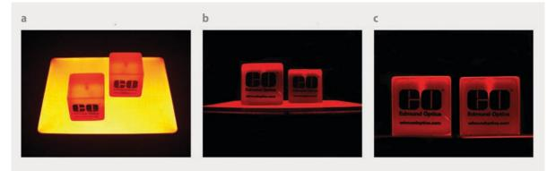
**Fig. 1** The two cubes are identical, but have different distances to the camera (a). Due to the aperture angle of the fixed focal length lens, the right cube is imaged smaller than the cube that is closer to the inspection system (b). In the same scene taken with a telecentric lens both cubes are the same size (c).
