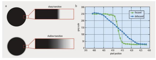
**Fig. 2** A telecentric lens depicts a point differently measured in focus (a, above) or with a slight defocus (below). The effect of defocus is distributed symmetrically. The course of the grey scale (b) shows that the edge is distributed over several pixels in the defocused case (blue), which can lead to more repeatable results than in the focused case (green).
