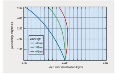
**Fig. 3** The example of a 1X lens shows that image height and telecentricity depend on each other differently at varying wavelengths.
