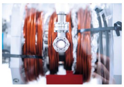
Fig. 2 Electron beam ion sources are direct sources of highly charged ions.
