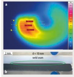
**Fig. 4** A thermal camera (a) proves the optimized energy input at a curve radius of 10 mm. The cross-section of the weld (b) shows its quality.
