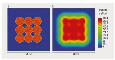
**Fig. 2** Spot shape at the focal plane (a) and at the working plane (b), where the spots overlap.
