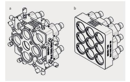
**Fig. 3** A multispot lens is available with (a) and without (b) possible adjustment of the *x*-*y*-position.
