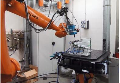
Multispot welding head during operation
