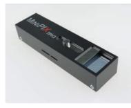
particle physics. The current "Timepix3" sensors allow a time resolution of 1.6 ns without any dead time at a count rate of up to 40 million events per second. The comprehensive "Pixel Pro" software supports the user in data acquisition and analysis. **Applications** include non-destructive fluoroscopy, X-ray imaging of tissue and animals, rock samples from geology, and crystal structure analysis using X-ray diffraction. Methods that require energy-re-
