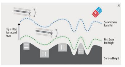
**Fig. 1** Magnetic Force Microscopy detects the sample topography in the first pass and the magnetic structure in the second pass [8].
