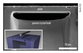
**Fig. 3** Thin plates of Mn<sub>1.4</sub>PtSn with defined thickness were extracted from a single crystal.
