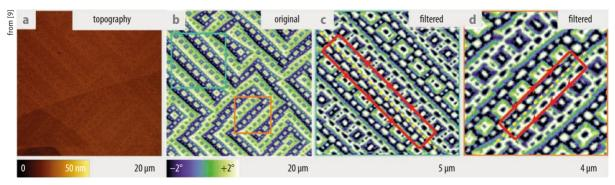
Fig. 2 The sample topography (a) shows a smooth surface. MFM measurements reveal more and more details with increasing magnification (b to d).
