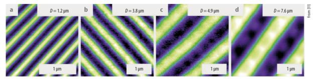
Fig. 4 With decreasing thickness (a to d), samples of Mn<sub>1.4</sub>PtSn show simple patterns of nested magnetic domains.
