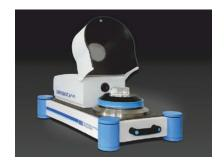
collimation image allows a fully automatic measurement with a very low measurement uncertainty. By evaluation of the autocollimation image and the angle value of the encoder in 3D space ("virtual tilting table"), the time-consuming adjustment of the spec-
