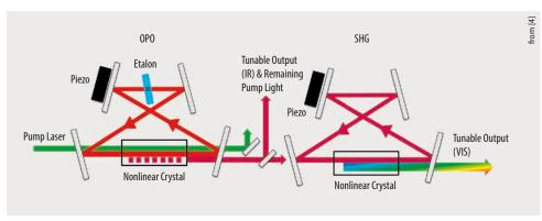
**Fig. 1** In a first step, a 532 nm laser pumps a nonlinear crystal to generate signal and idler photons (the range 900 – 1300 nm). Wavelength selection and subsequent second harmonic generation (SHG) converts either signal or idler photons into the visible range of the spectrum (450 – 650 nm). The green arrow depicts the pump laser beam, dark red and light red arrows depict the signal respectively the idler beam (arbitrary assignment).
