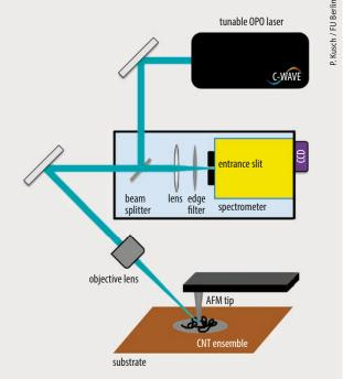
**Fig. 3** A fully tunable OPO laser is guided through a beam splitter and focused onto the tip of an atomic force microscope probe. Spectra are recorded by guiding the tip-enhanced Raman scattered light of the sample into a grating spectrometer.
