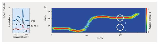
**Fig. 4** (a) Composed (blue line), far-field (black line) and tip-enhanced Raman spectra (red line) of the radial breathing modes of several carbon nanotube species. The tip-enhanced Raman spectrum can be unambiguously assigned to a nanotube of (7,5) chirality. (b) Nanoimage of the (7,5) carbon nanotube, obtained by plotting the tip enhanced RBM intensity as a function of tip position.
