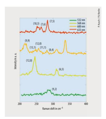
**Fig. 2** Resonance Raman scattering spectra of a mixture of single-wall carbon nanotubes (CNTs) in ethanol solution (concentration of 1 g/l). The spectra are recorded for excitation wavelengths of 633 nm, 600 nm, 568 nm, and 532 nm (from top to bottom). The peak captions indicate the peak assignment to signals of CNTs of a particular chirality (n,m).
