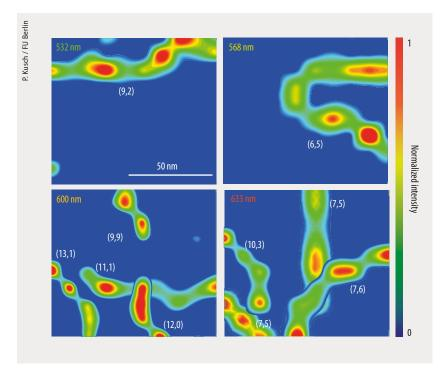
**Fig. 5** Nanoimages of carbon nanotubes recorded with four different excitation wavelengths. The different tube species are labeled by their chiral indices in the nanoimages.
