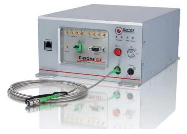
**Fig. 4** iChrome CLE, standard configuration 405, 488, 561, 640 nm with 20 mW per wavelength delivered via a single-mode fiber optic
