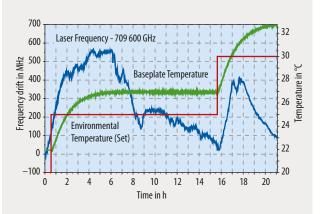
**Fig. 3** Frequency of a DLC MDL pro laser at 423 nm exposed to two temperature steps of 5 °C. The measured frequency drift of 550 MHz is significantly lower than the mode-hop-free tuning range of 30 GHz. Even under these conditions, active feedback will keep the laser on resonance.
