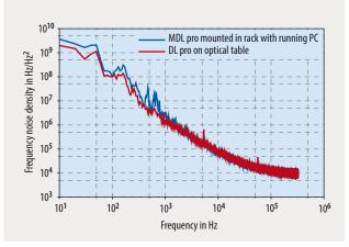
**Fig. 2** Comparison of frequency noise density: a DLC MDL pro installed in a rack along with an air-cooled computer compared to a DL pro mounted on an optical table. The increased noise is at low frequencies so that feedback for correcting these requires only little effort.
