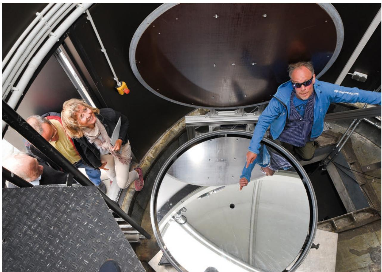
**Fig. 3** Far-field detection uses a 1.5 meter diameter primary mirror for efficient signal collection. Left to right: Thomas Trickl (KIT), Ulrich Emmerichs (Coherent), Petra Wallenta (Coherent), Hannes Vogelmann (KIT) – project meeting at mount Zugspitze (2.962 m). UV-Coherent-Laser successfully works there for climate research.
