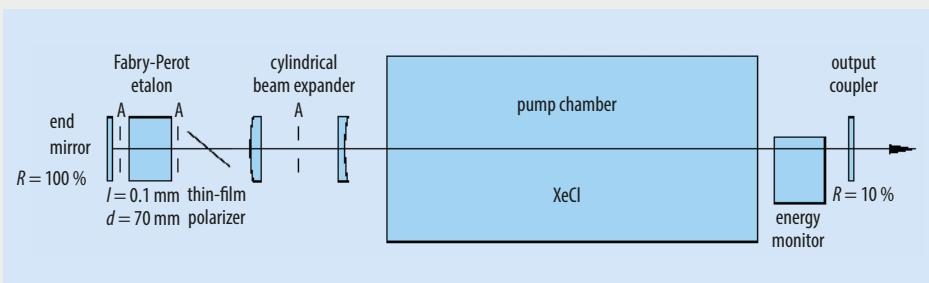
**Fig. 2** Scheme of the modified laser system; A: sand-blasted aluminum apertures [4].
