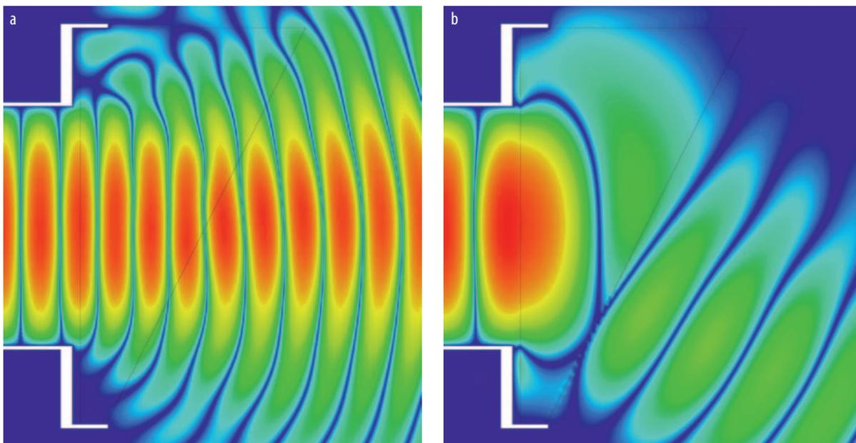
Fig. 4 Electric field values in the metamaterial wedge lens from Fig. 3, (left) in the double-positive region and (right) in the double-negative region.
