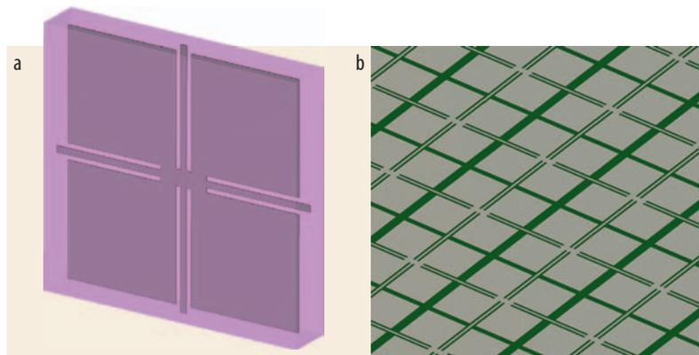
Fig. 1 A single gapped plane element (a). An EBG power plane for a low-noise PCB (b).
