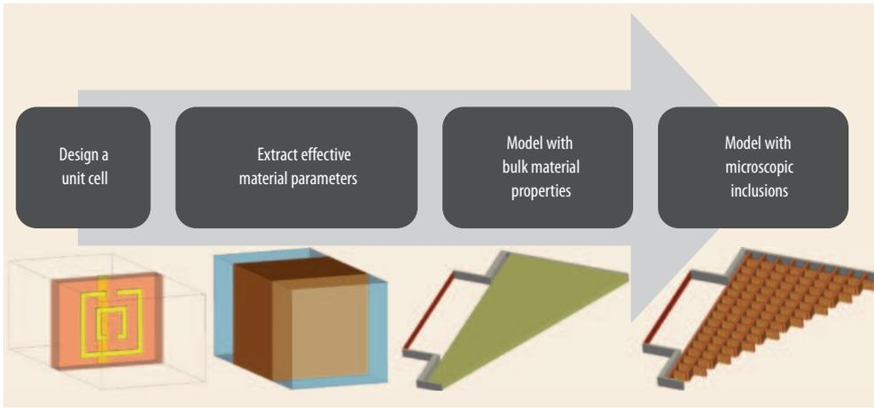
Fig. 3 Workflow for modeling the behavior of a metamaterial system, from a single unit cell to a whole device.
