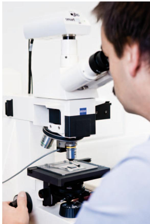
Fig. 1 Most microscopes of well known suppliers can in principle be extended without many complications. The interference lens is one of the central elements of the extension. A table that moves the sample in *xy*-direction allows scanning large regions of a structured surface in a very short time span.
